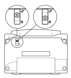
Your scanner has a locking mechanism to protect it during shipment or while you move it
